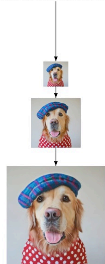
Figure A.4: Visualization of Imagen. Imagen uses a frozen text encoder to encode the input text into text embeddings. A conditional diffusion model maps the text embedding into a 64 \times 64 image. Imagen further utilizes text-conditional super-resolution diffusion models to upsample the image, first 64 \times 64 \rightarrow 256 \times 256 , and then 256 \times 256 \rightarrow 1024 \times 1024 .
