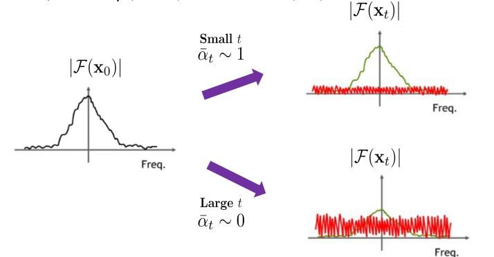
In the forward diffusion, the high frequency content is perturbed faster.
