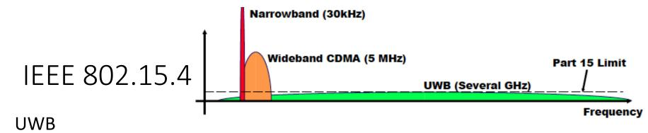
Uses more bandwidth than the minimum required for the signal transmission (SS) BUT
