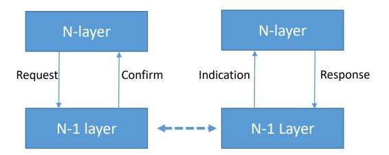
**Request**: The request primitive is passed from the N-th layer to the (N-1)-th layer to request that a service is initiated. *e.g. a node creates a MAC packet @ the MAC layer*  $\rightarrow$  *PHY Layer*
