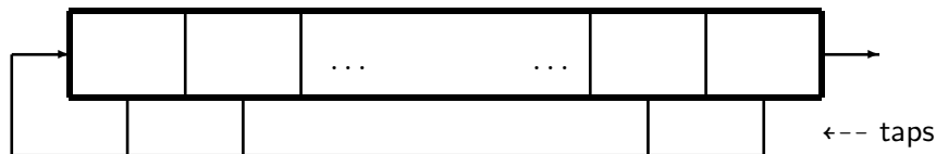
Figure 8.23: Simple graphical representation of an LFSR
